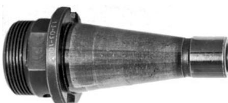
If the toolholder shows a wear pattern in two areas one at the gage line and the other at the small end of the taper, the toolholder does not fit the spindle.
