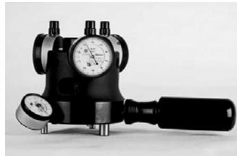
JM Performance Products used the Taper Shank Test Fixture to test different retention knobs and toolholders on the market. JMPP was able to prove that standard retention knobs made to any of the 5 world standards, expand the toolholder shank at the small end when tightened to an adequate torque pressure.
